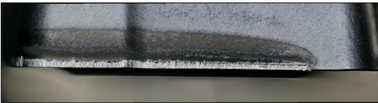
Left: Light optical microscopy image of cutting insert. Right: Associated mask with two types of wear marked in blue and yellow
