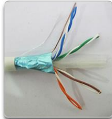
Shielded Twisted-Pair (STP) cable
