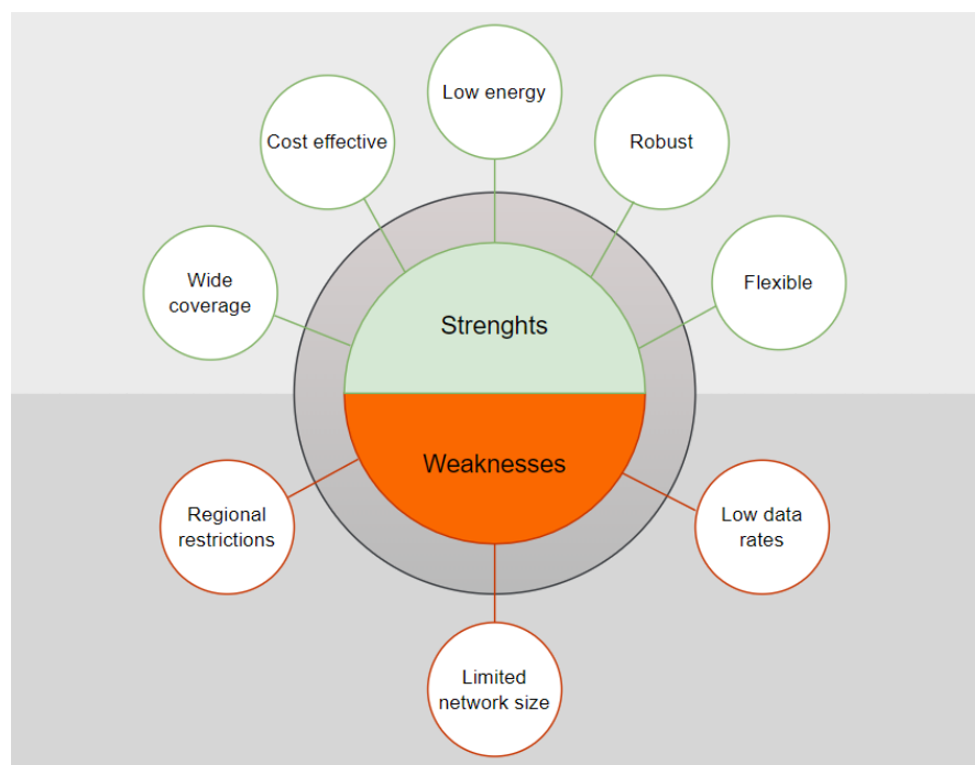
Figure 2.5 Illustration of strengths and weaknesses of LoRa and LoRaWAN
