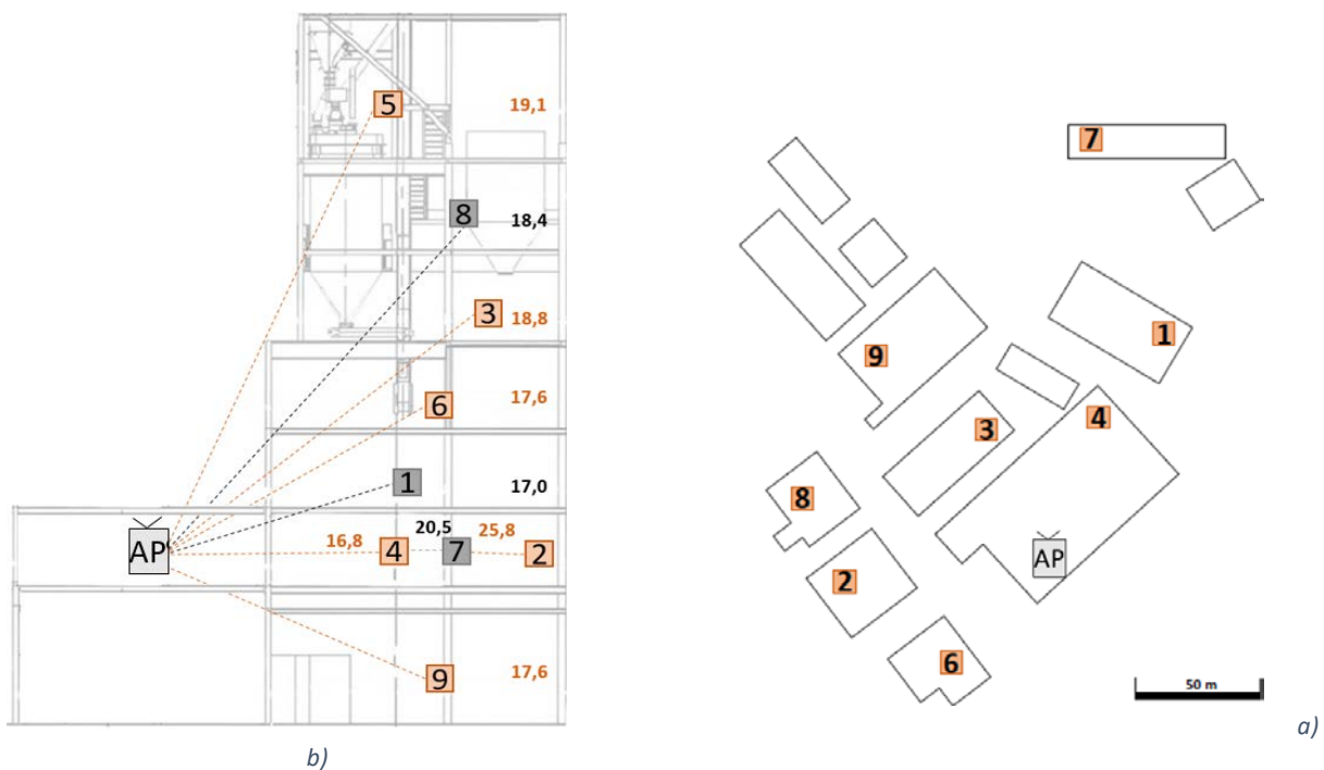
Figure 2.18 Layout of the measurements: a) scenarios 1 and 2, b) scenario 3
